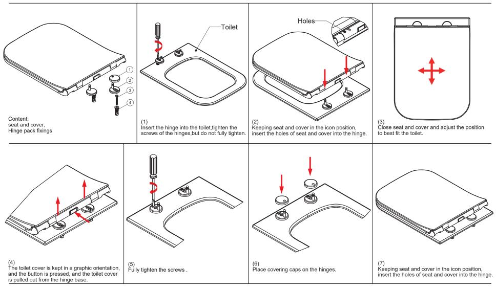
\*\*Important:Do not over tighten the nuts as this could crack the toilet bowl.
