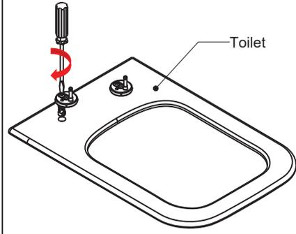
(1) Insert the hinge into the toilet, tighten the screws of the hinges, but do not fully tighten.
