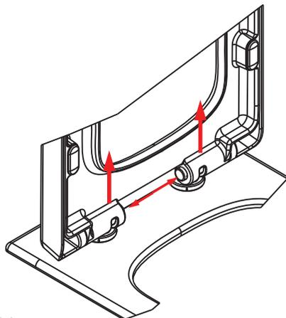
(4) The toilet cover is kept in a graphic orientation, and the button is pressed, and the toilet cover is pulled out from the hinge base.
