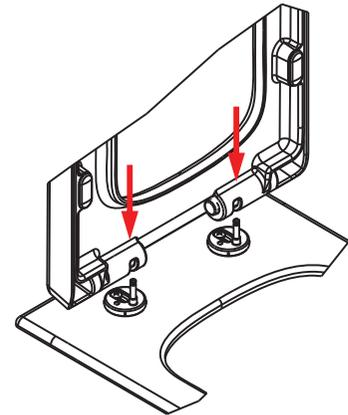
(2) Keeping seat and cover in the icon position, insert the holes of seat and cover into the hinge.
