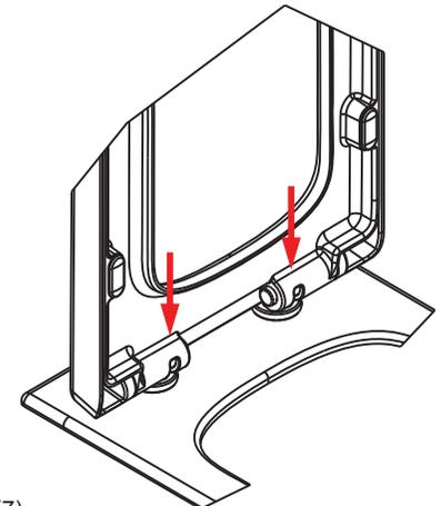
(7) Keeping seat and cover in the icon position, insert the holes of seat and cover into the hinge.
