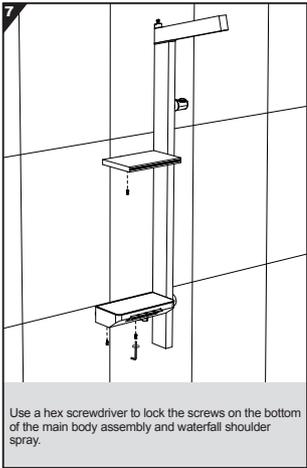
Use a hex screwdriver to lock the screws on the bottom of the main body assembly and waterfall shoulder spray.
