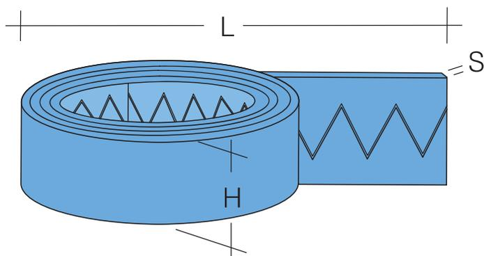
PROTEZIONE ANTIURTO E ACUSTICA AUTOADESIVA A ZIG-ZAG PER TUTTE LE TIPOLOGIE DI SANITARI ES: WC E BIDET A PAVIMENTO E SOSPESO, LAVABI A COLONNA E CONSOLLE, SOPRA E SOTTO PIANO, CASSETTE A ZAINO, ORINATOI ECC. ECC.
